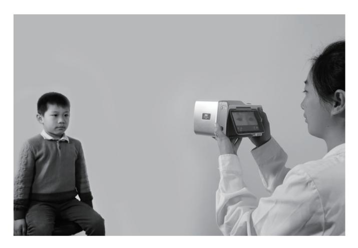
The Cell vision screener V100 is a portable diagnostic device designed for clinicians to quickly detect vision abnormalities on patients from 6-month old to adults. Cell can screen both eyes at once from a distance of 1 meter. Once the pupils are in focus, the device will start to calculate automatically and deliver results within 1 second. The touch screen allows users to operate conveniently like using a smart phone.
